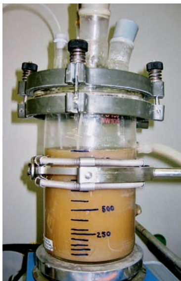
Murky mixture: Magnesium-chloride is added to urine (Photo Yvonne Lehnhard)
