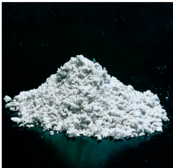
Clean product: A pure nutrient powder is obtained (urine-based fertilizer struvite) (Photo Mariska Ronteltap)
